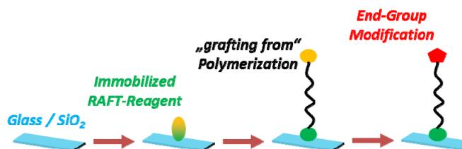
**Figure 3:** Step-by-step strategy for the preparation of RAFT polymer brush coatings on silicon oxide substrates
