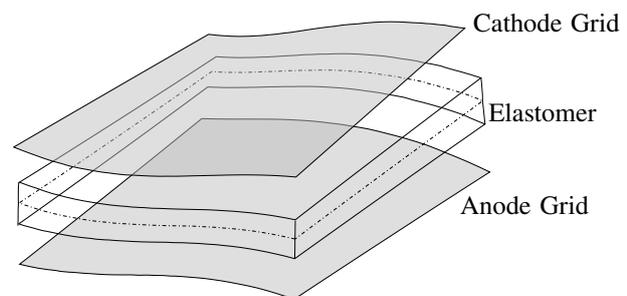
**Figure 1:** Construction of an electro-active elastomer actuator.
