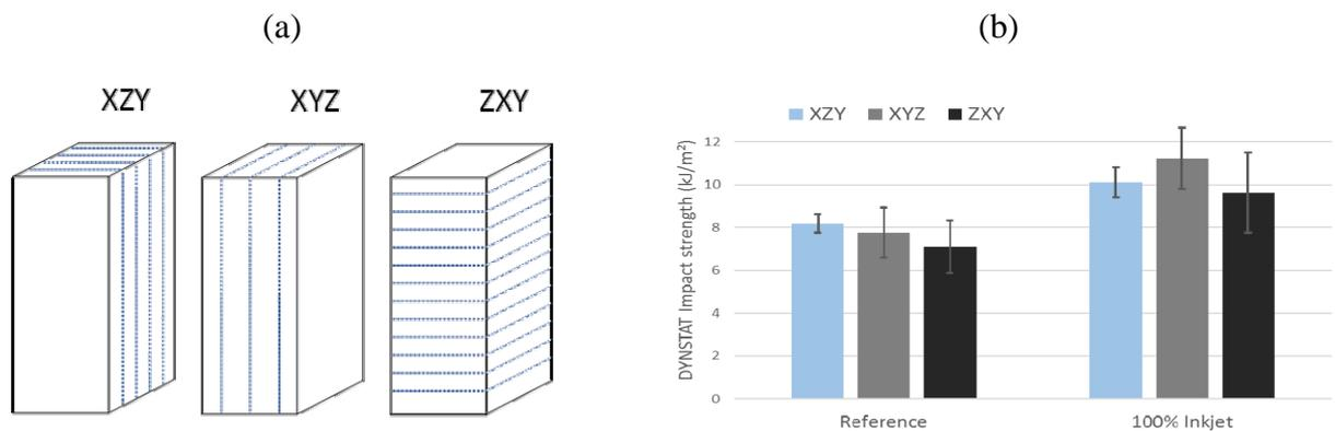
**Chart 2** Different jetting directions, correlating the building direction of the printed part (a). In each direction, a significant increase of the impact strength was observed (b)
