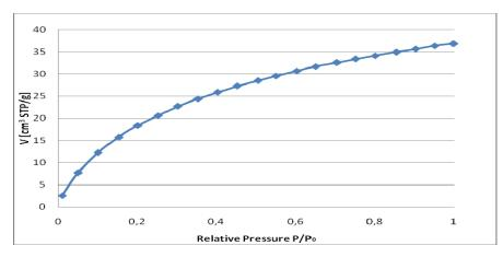
Fig 2. Isotherms of CO2 adsorption on activated lignite
